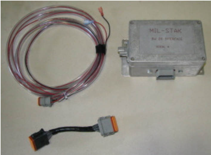
BW 28 Interface & Wire Harness Part # 1P7510 (pre automation) limited availability.
